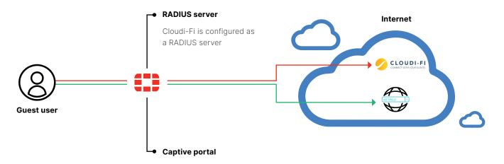
Enable the **RADIUS Authentication** and configure the **redirect host** with a **FQDN** returning the **Fortinet Captive Portal Redirect IP**
